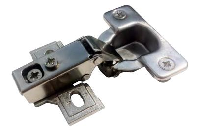
Concealed euro-style face frame cabinet hinge, self-closing, 1/2" overlay, wrought steel, with cast zinc mounting plate, nickel plated. Unique design eliminates the large gap between the door and face frame. 125\* opening angle.
