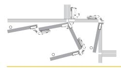
At the start of its swing, the door element opens about 50° on the handle side.
