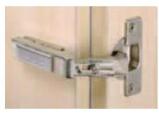
Concealed hinge, snap-on assembly, integrated door overlay and eccentric depth adjustment Opening angle 50°/90°, cup diameter 35 mm
